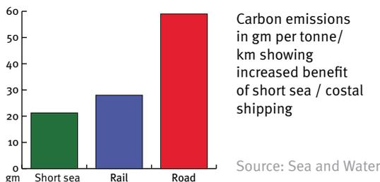
A 1000 tonne coaster typically uses a 600hp engine and steams at about 10 knots, burning about 5 litres of marine diesel oil per kilometre. An HGV typically carries 30 tonnes, uses a 500hp engine and burns about 0.4 litres of diesel per kilometre.
